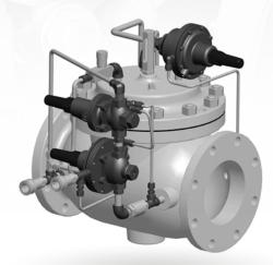
The OCV Model 114-3 is a control valve specifically designed for aircraft refueling service. Known as either a refueling or a hydrant control valve, it is the typical control valve used on pantograph refueling systems. It opens and closes via hydraulic deadman control, modulates to control downstream pressure at a predetermined set point whole open, and closes rapidly to prevent undue pressure buildup due to a rapid reduction in demand (HCV).
